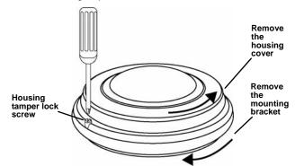
Figure 2 Remove the housing cover and mounting bracket 2. Install the battery included with the unit.
