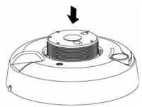
Figure 5 Push down on the optical chamber
